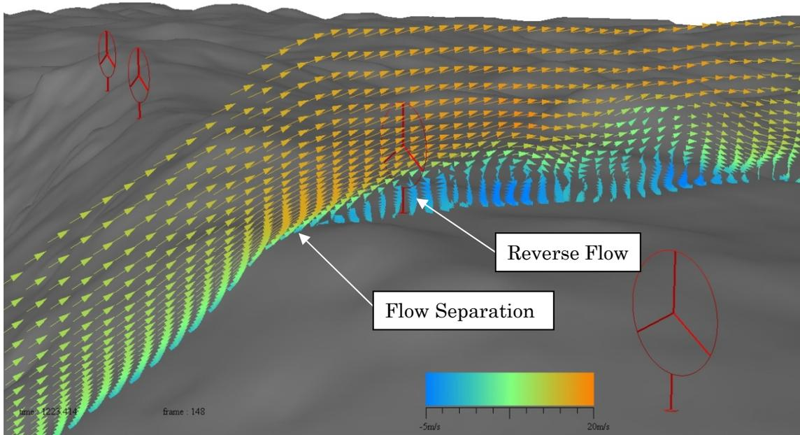
Fig.3 - Instantaneous vector plot at turbine T12
