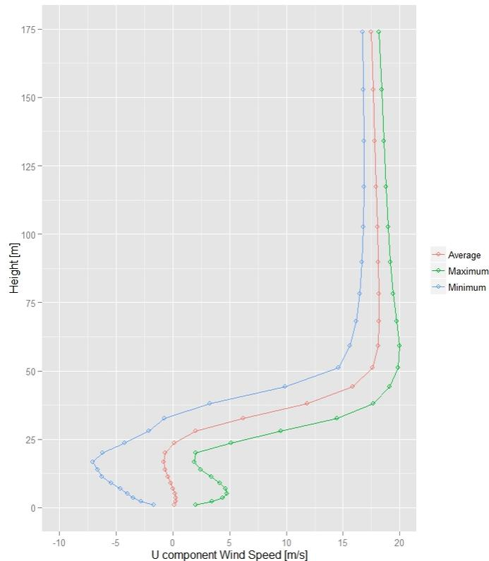
Fig.5 - Vertical Shear Profile predicted by RIAM-COMAPCT®
