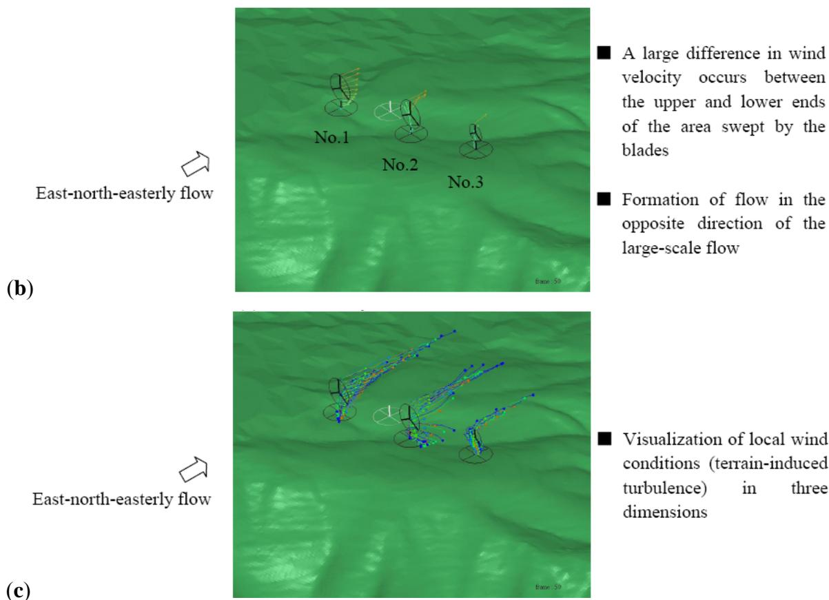
The unexpected large differences in the wind velocity across heights may induce vibrations of the WTGs and may also cause internal damage and breakage of the WTGs. Deployment of virtual particles and examination of the trajectories of these particles are an effective method for the assessment of the three-dimensional wind conditions at a site of interest. Figure 8c vividly shows the three dimensional structure of the terrain-induced turbulence discussed above.
